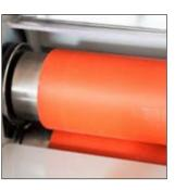
distance of roller adjustable (max. 6 mm)
