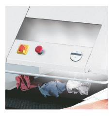
**ILLUMINATION OF THE WORKING AREA** The feeding area and the conveyor belt are illuminated by LEDs.
