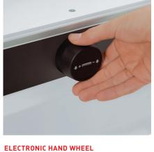
Ideal for manual backgauge positioning, the electronic hand wheel has infinitely variable speed control from very slow to very fast.
